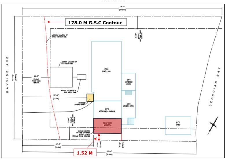
Proposed Attached Garage Addition Proposed Covered Entry
